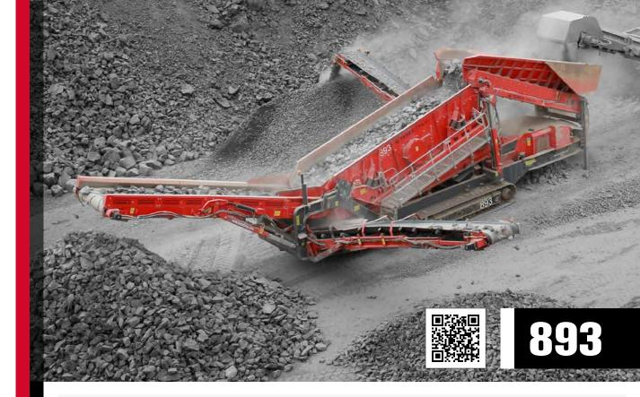
The Terex Finlay 893 heavy duty screen is a robust high capacity machine, engineered and built for working in quarrying, mining, construction and demolition debris, topsoil, recycling, sand, gravel, coal and aggregate applications. The 893 features an aggressive forward-facing inclined modular configuration screen box with a 6.1m x 1.83m (20' x 6') top deck and a 5.5m x 1.83m (18' x 6') bottom deck and can accept bofar bars, speedharps, woven mesh, punch plate, tines and cascade fingers.
