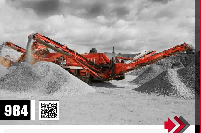
The Terex Finlay 984 is a high performance horizontal 3 deck screener that is easy to set up, versatile and ideal for handling large volumes of material in quarrying, mining and recycling applications.
