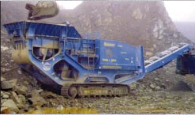
1100x800 Premiertrak crushing blasted hard rock.
