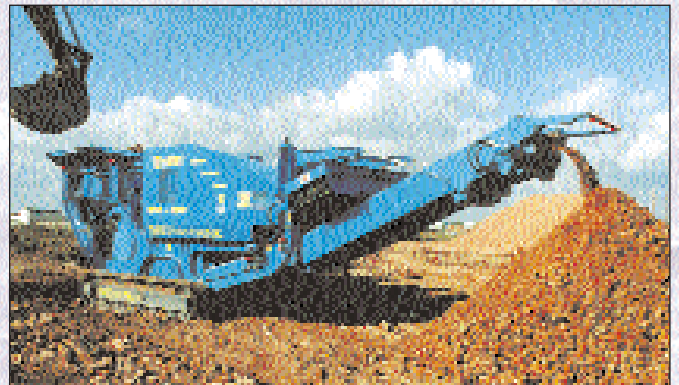
Metrotrak recycling brick rubble.
