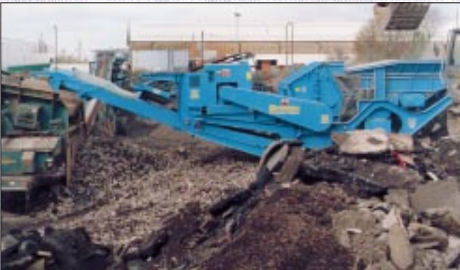
428 Trakpactor recycling concrete and asphalt
