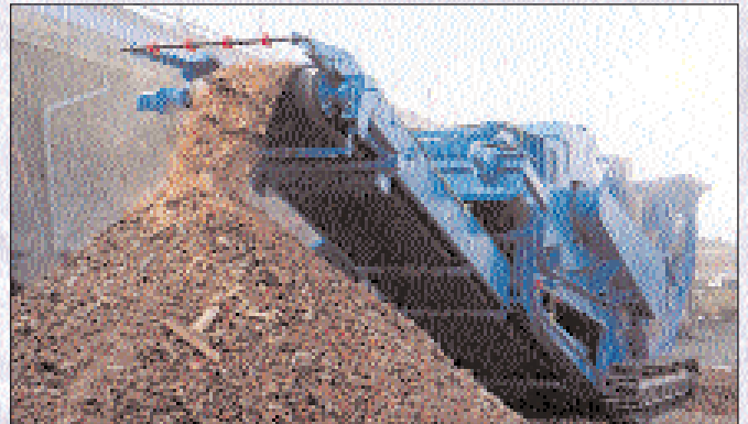
428 Trakpactor recycling construction and demolition waste.
